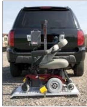
Loaded product secured and ready for lifting.
